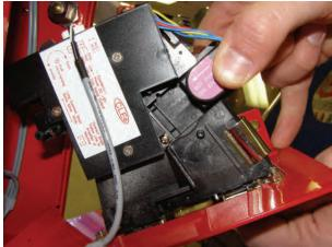
STEP 2: Pull back the coin holder and insert your coin into the coin slot.
