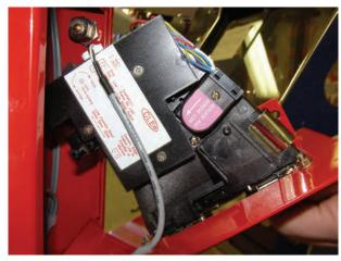
STEP 1: At each station open the coin door to access the coin comparator.
